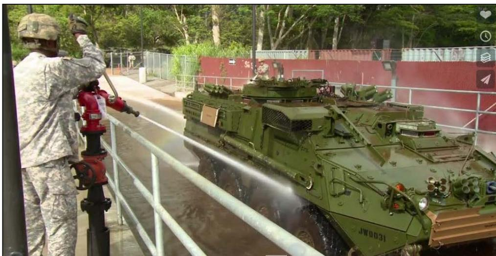
**Figure 7.** Still from the CVWF video, showing soldiers cleaning a stryker with water cannons during the pre-wash bath.
