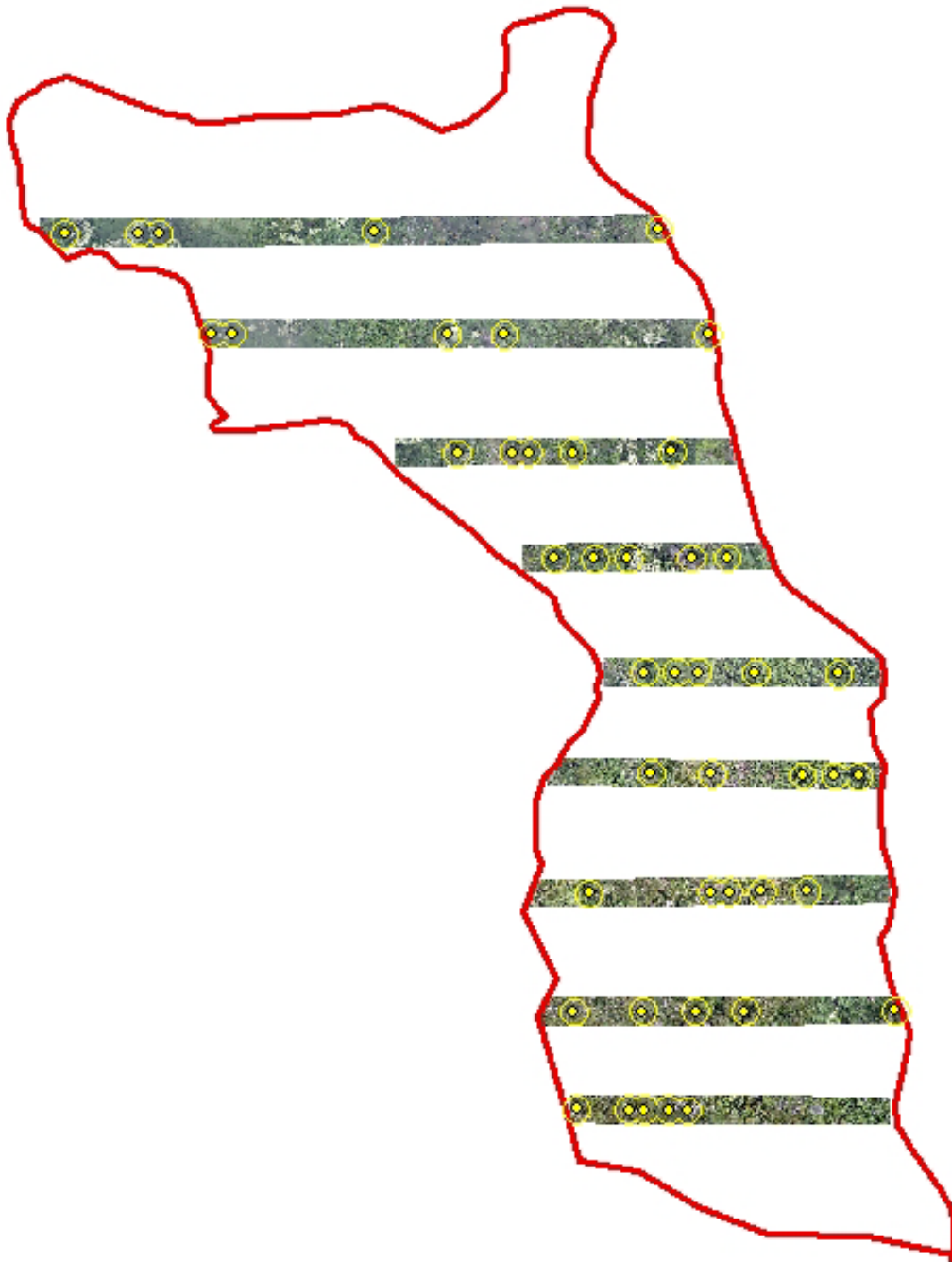
Figure 35. UAS image transect example for Kahanahaiki with random 20 meter diameter plots.
