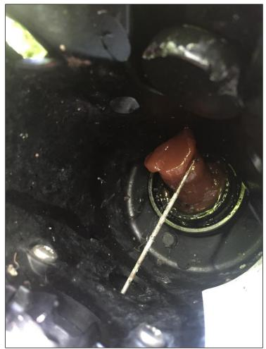
Figure 12: Auto lure baiting device installed and functioning in A24 trap.
