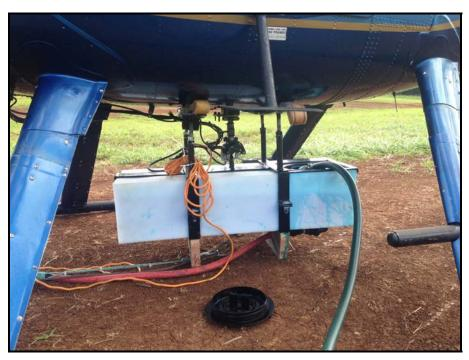
Above: the spray rig is attached to the helicopter via the belly hook and cushioning arms. The light colored tank allows staff to gauge how much spray mix is left. A large top port allows for easy filling.
