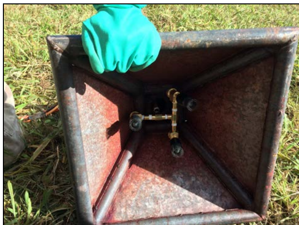
Left: array of three 'rain' nozzles. Right: spray ball with 'rain' nozzles being tested prior to flight.
